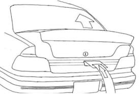
•BEFORE INSTALLING RACK ON VEHICLE, REMOVE BOTTOM STRAPS OPEN TRUNK SLIGHTLY AND PLACE BOTTOM HOOKS JUST INSIDE OF TRUNK/HATCH. CAREFULLY CLOSE TRUNK ON BOTTOM STRAP. PULL STRAPS TO BRING HOOKS AGAINST THE INSIDE
