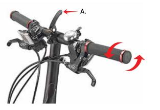
**NOTE:** Remember to rotate the handlebars back up per step 3B to achieve the correct brake angle when unfolding your bicycle.
