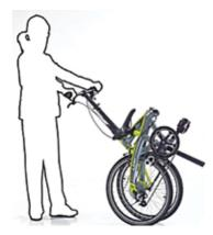
**C.** To release the locking wheels, either lift or push down the locking tab.
