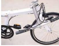
7. Fix handlebar with the frame strap a) Use the strap to fix the wheels and the handlebar post.
