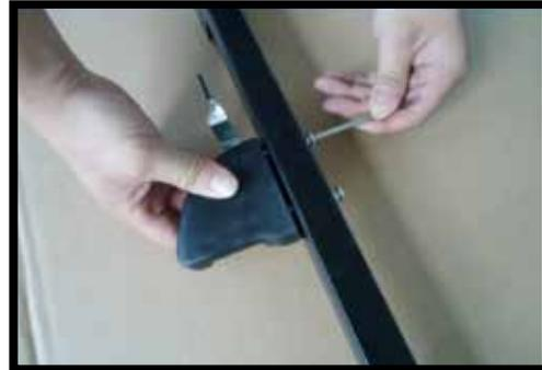
**STEP 4:** Place the Wheel Guard/Brake Assembly against the frame, and use the hex key wrench provided to tighten the screws until snug.
