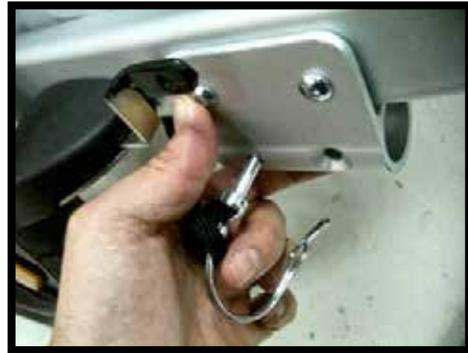
**STEP 2:** Next, take one arm, ( Right and left arms are not the same, note the screw thread faces up), insert into the aluminum bracket, align with the fixing hole and insert and lock the spring pin.
