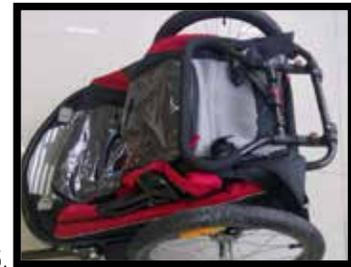
**NOTE:** The trailer can be folded with or without the wheels on. If the wheels are removed, they can be stowed inside the trailer when not in use. To remove the wheels, simply push the button in the wheel, and pull the wheel out from the frame.
